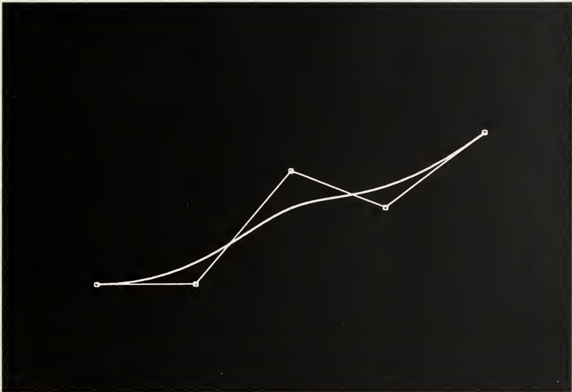
Fig. 8. Fourth order B-spline curve.
